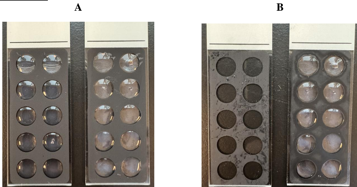
Figure 1: Firm Attachment of Agarose Gel on CometCoat™-Treated Slides. A: Solidified agarose gels containing cells on untreated (left) and CometCoat™-treated (right) 10-well glass slide. B: After cell lysis, alkaline treatment and electrophoresis, agarose gels detached from the control slide (left), and remained firmly attached the CometCoat™-treated slide (right).
