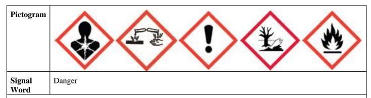
**Hazard Statements:** Highly flammable liquid and vapour (H225), Harmful if swallowed (H302), Causes serious eye damage (H318), Causes serious eye irritation (H319), Suspected of causing cancer (H351), Very toxic to aquatic life with long lasting effects (H410).
