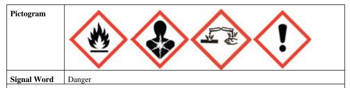
**Hazard Statements:** Flammable solid (H228), Harmful if swallowed or inhaled (H302 + H332), Causes skin irritation (H315), May cause an allergic skin reaction (H317), Causes serious eye damage (H318), May cause respiratory irritation (H335), Suspected of causing cancer (H351), Harmful to aquatic life with long lasting effects (H412).
